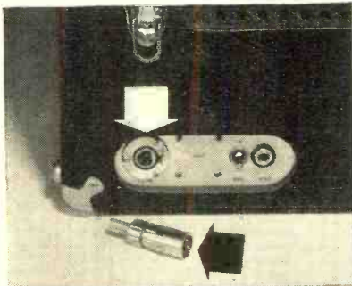
Arrows point to XL Plug and Receptacle
