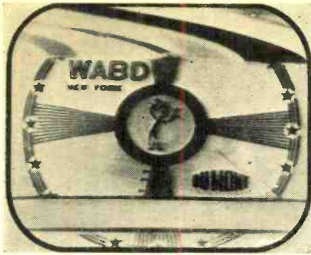
Fig. 1. A typical case of "tearing" which may result from several different receiver faults. The strip near the bottom is not tearing but is a news ticker strip which is part of test pattern being transmitted.
