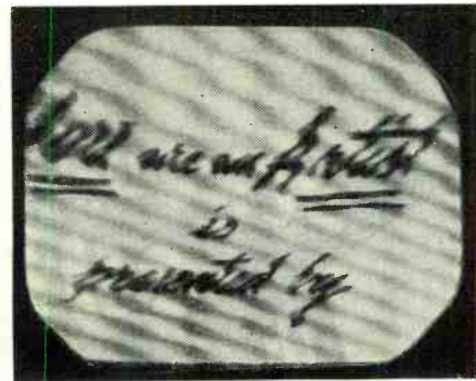
Fig. 18. Another example of FM interference with modulation pattern in evidence.
