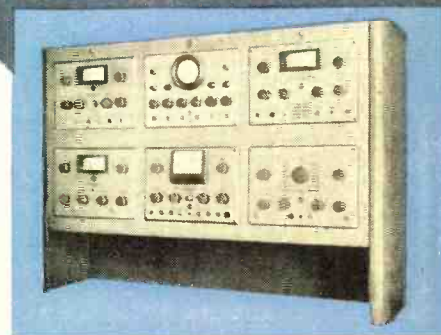
Complete TV/FM/AM Service set-up with RCA matched test units
