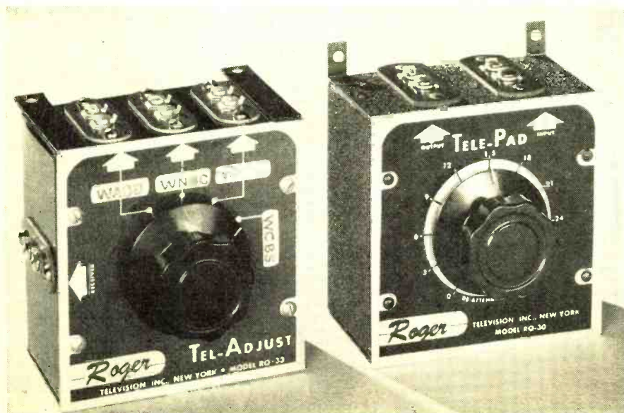
Fig. 9. (Left) Signal selector and equalizer box with cover and knob in place. Station call letters are inscribed in ink or pencil for home or tavern installations. For dealer store demonstration setups, receiver model numbers may be written in instead of calls. (Right) A commercially-built variable pad box for TV installations.
