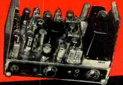
Typical Motorola FM two-way radiotelephone receiver utilizing Sealed in Steel Chicago Transformers.
