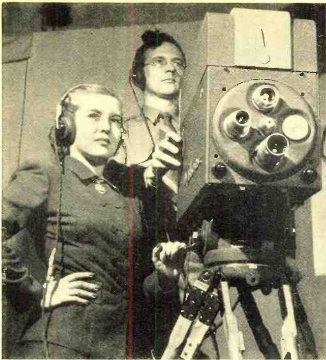
Commercial video broadcast equipment at American Television, Inc., includes the latest RCA image orthicon camera links as well as iconoscope cameras for studio use by the trainees.
